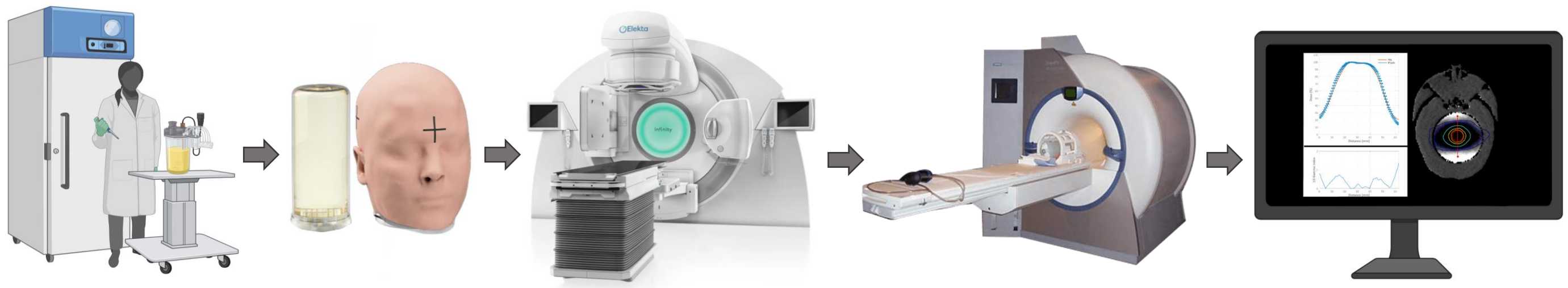
Figure 3. Step-by-Step Workflow from VIPET Polymer Gel Production to Dose Readout and Gamma Index Analysis.
