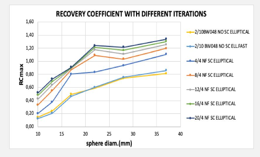
1 RC<sub>max</sub> values for the 22 mm sphere showed a relative increase of 30% when iterations were increased from 4 to 8, 13% for 8 to 16 iterations and 2% for 16 to 20 iterations.
