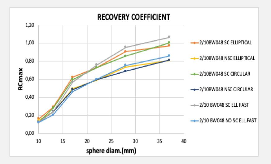
1 RC decreases with the diameter of the spheres (due to PVE).
