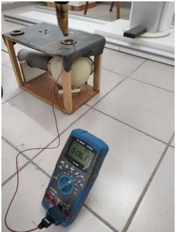
The efficiency of a scintillator to emit light, after X-ray exposure, can be experimentally determined under clinical conditions by the absolute luminescence efficiency (AE), defined in terms of emitted light energy flux ( $\Psi_{\lambda}$ ) per unit of incident exposure rate, i.e. (Michail et al., 2019):
