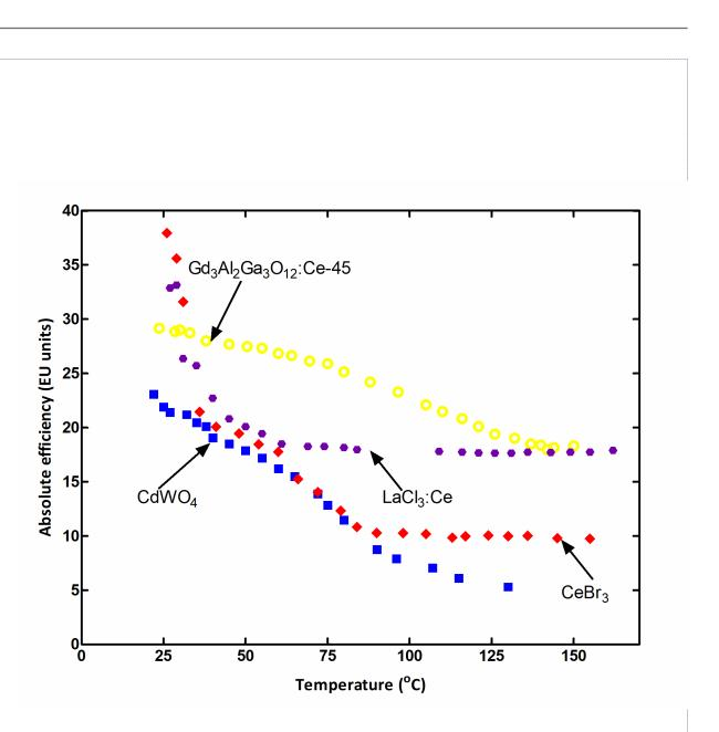
Data on the thermal behavior of scintillators, such as GAGG:Ce is useful for various applications, from medical imaging up to detectors for extreme environments.
